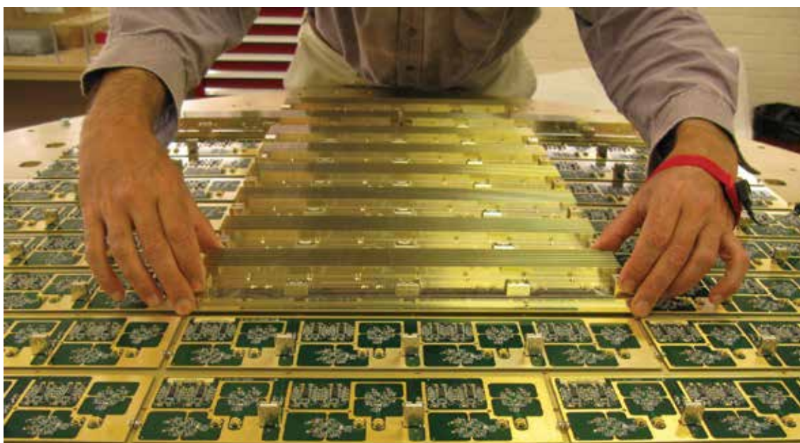
Installing shields to prevent radio frequency interference from affecting the signals collected by CSIRO's ASKAP antennas (Courtesy of the CSIRO, credit Russ Bolton)
